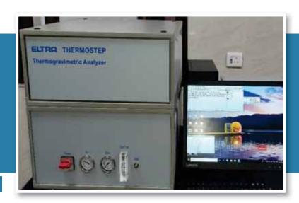
Thermogravimetry (TGA) is a technique that measures the change in weight of a sample as it is heated, cooled or held at constant temperature. Its main use is to characterize materials with regard to their composition. Application areas include plastics, elastomers and thermosets, mineral compounds etc.
