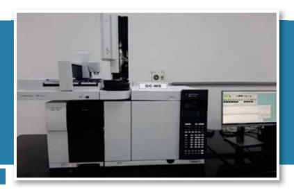
GC-MS is the analytical technique of choice for smaller and volatile molecules. It is mainly used to identify and quantify narcotics, drugs, psychotropic substances, pesticides, pharmaceuticals, hazardous chemicals, etc.
