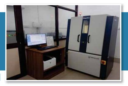
X-ray Diffractometer (XRD) is used to determine the atomic and molecular structure of a crystal/powder, in which the crystalline structure causes a beam of incident X-rays to diffract into specific directions. By measuring the angles and intensity of these diffracted beams, identification of the minerals is carried out.
