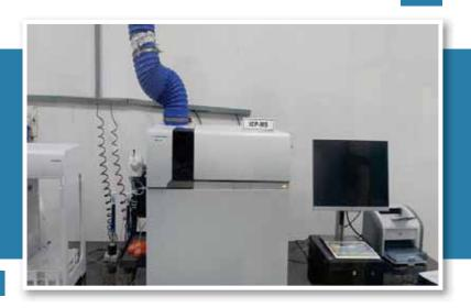
Inductively coupled plasma mass spectrometry (ICP-MS) atomizes the sample and creates atomic and small polyatomic ions, which are then detected by mass spectrometer. It can detect metals and several non-metals at very low concentrations i.e. PPB (Parts Per Billion). It can also detect different isotopes of the same element. It is used for simultaneous determination of elements in one test.
