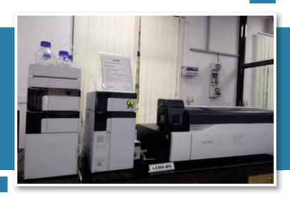
Liquid Chromatography with tandem mass spectrometry (LC-MS-MS) is a powerful analytical technique that combines the separating power of liquid chromatography with the highly sensitive and selective mass analysis capability of triple quadrupole mass spectrometry. Identification and quantification by this instrument is mandatory under FSSAI regulations in toxic and residual organic compounds in food.
