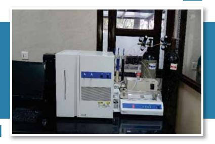
AOX/TOX analyzer is used to detect all organic halides i.e. chlorine, bromine & iodine in the samples of Waste oil/Used oil, by coulometric titration, as per ASTM/EPA test methods.
