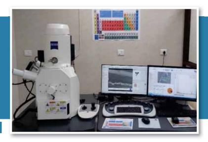
The scanning electron microscope (SEM–EDAX) is one of the most versatile instruments available for the examination and analysis of the microstructure & morphology. Analysis of chemical composition & characterization is also possible with EDAX.
