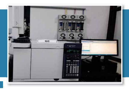
Gas chromatography (GC) is a common type of chromatography used in analytical chemistry for separating and analyzing compounds that can be vaporized without decomposition.
