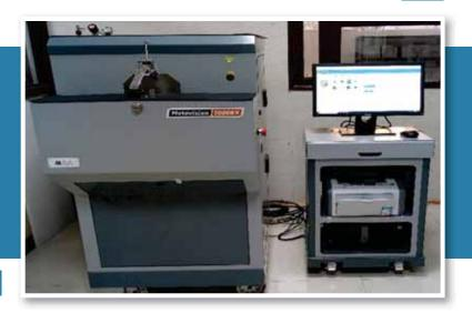
Optical Emission Spectroscopy (OES), is a well trusted and widely used analytical technique used to determine the elemental composition of a broad range of metals. The type of samples which can be tested using OES include samples of tubes, bolts, rods, wires, plates and many more.
