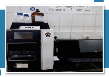
High-performance liquid chromatography (HPLC) is used to separate, identify, and quantify each constituent of a mixture of organic compounds. Availability of HPLC has enabled some of the Revenue Laboratories to obtain NABL accreditation for testing of azo dyes.
