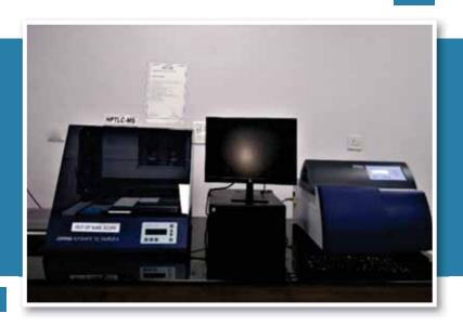
This equipment is the most advanced form of Thin Layer Chromatography. Further coupling of High Performance Thin Layer Chromatography with Mass Spectrometry provides a high degree of sensitivity and accuracy in analysis of samples.
