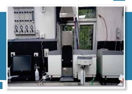
Atomic Absorption Spectrometry (AAS) is an analytical technique that measures the concentrations of elements. The technique makes use of the wavelengths of light specifically absorbed by an element. Concentration of elements is measured at ppm (parts per million) levels.
